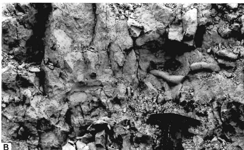
Fig.1. Examples of jointing in a Chalk rock-mass; (above) Turonian of Lincolnshire, "northern province" and (below) Turonian of Buckinghamshire, "southern province". (Photos by C.J. Wood.)
