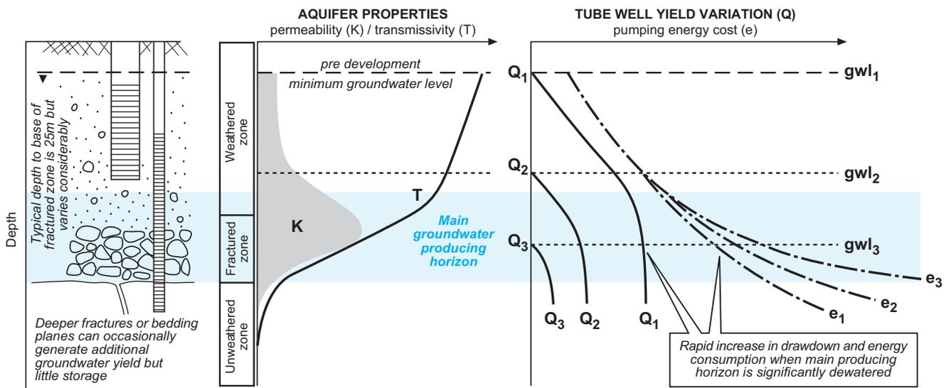
ESCALATING WATERWELL ENTRY LOSSES & UNIT ENERGY CONSUMPTION WITH DEWATERING OF A SHALLOW AQUIFER
